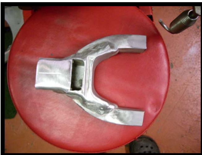
I Removed the 450 engine and welded an aluminum plate on top to cover the hole.
