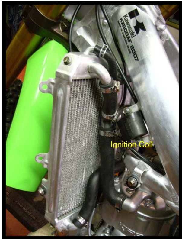
The mounting brackets for the coil welded in new place
