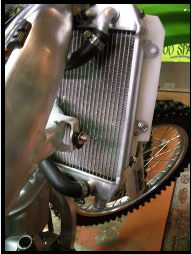
Right radiator with a new hose connector at the bottom The lower crossover have been re-angled
