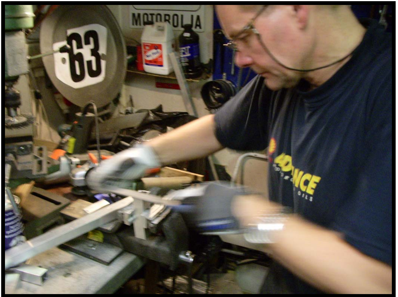
Rolle in the works of bending, twisting and fitting frame extensions out of 25x25x2 mm aluminum profile.
