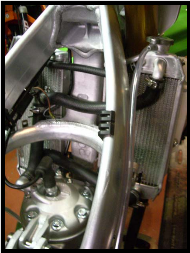
I used hoses from different sources, like pre bent car heater hoses
