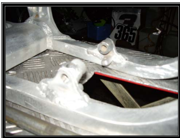
Lower engine mounts welded in new place
